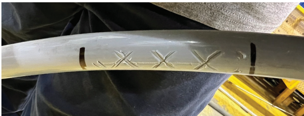
Figure 6-10: Sample 3.1.2 - 17 kV, 1/0 AWG ACSR Condition after Test
