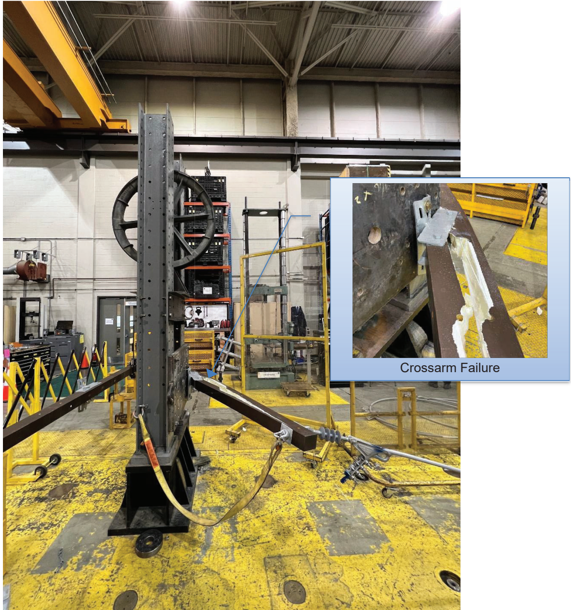
Figure 6-22: Sample 6.1 – Failure Location
