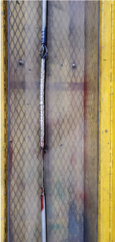
Figure 6-5: Sample 1.1.1 after test (conductor failed at South end of splice)
