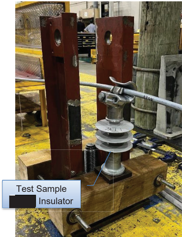
Figure 4-2: Clamp Slip Test Setup
