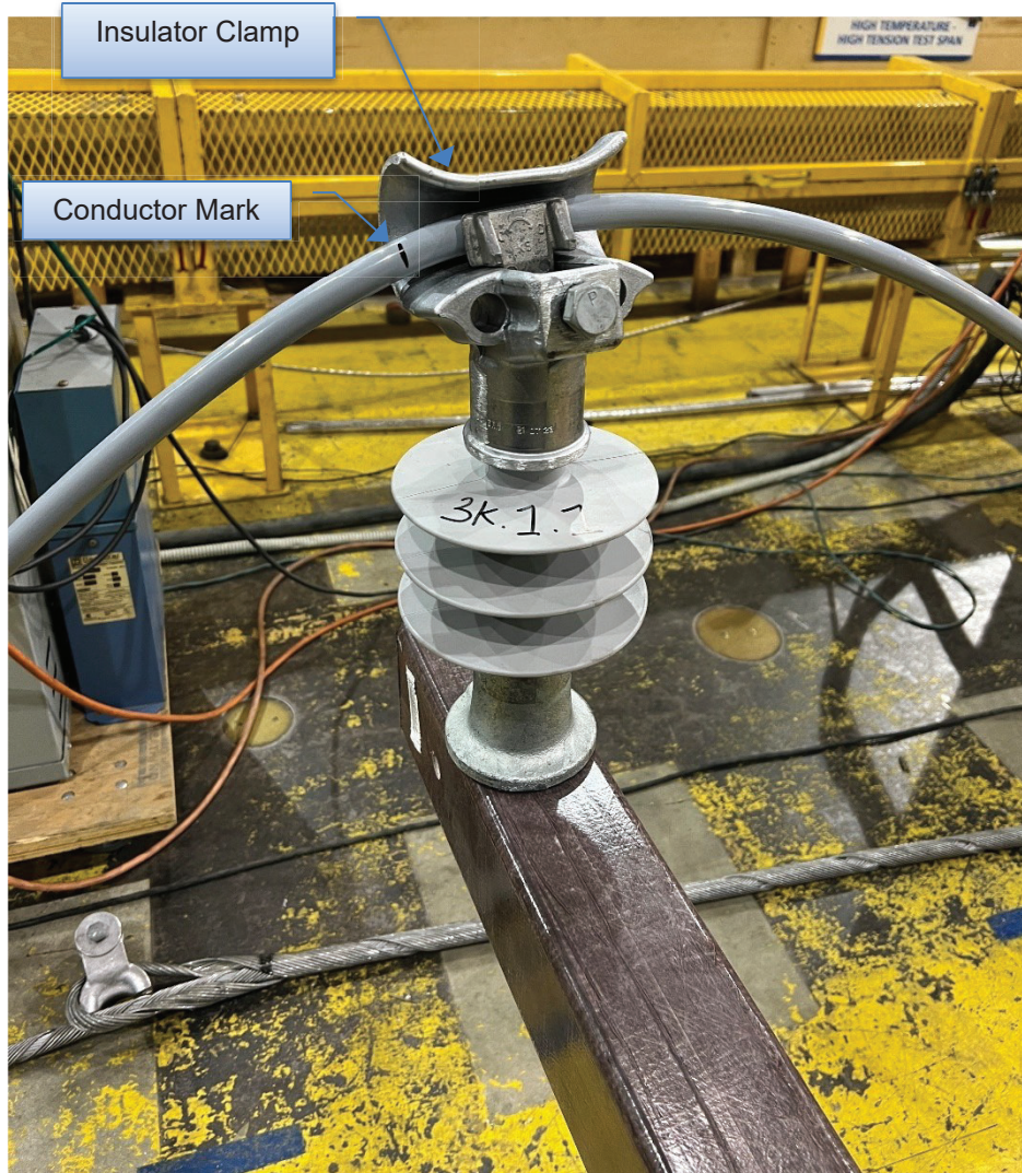
Figure 6-27: Sample 3K.1.2 – Insulator and Cross-arm Condition after Test
