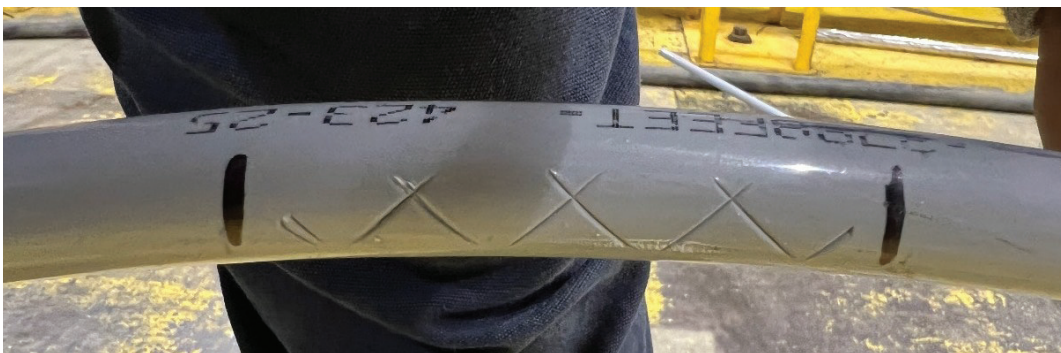
Figure 6-12: Sample 3.1.3 - 17 kV, 1/0 AWG ACSR Condition after Test
