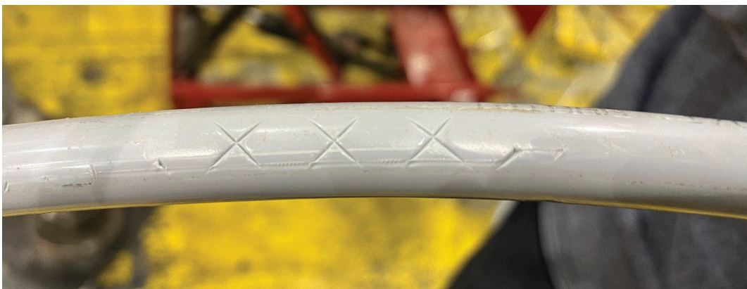
Figure 6-24: Sample 3.4.3 - 15 kV, 1/0 AWG ACSR Condition after Test
