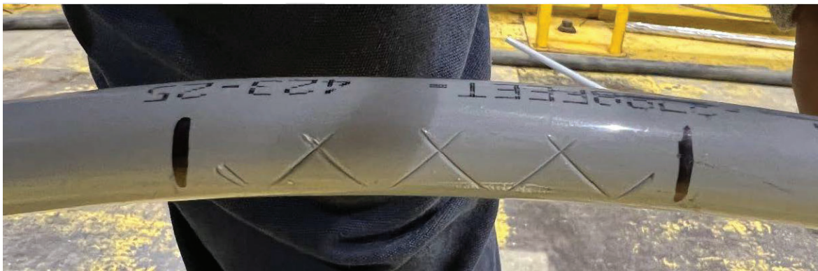
Figure 69. A representative post-test image showing superficial marks on the conductor at the vise-top insulator grip location (17-kV 1/0 ACSR).
