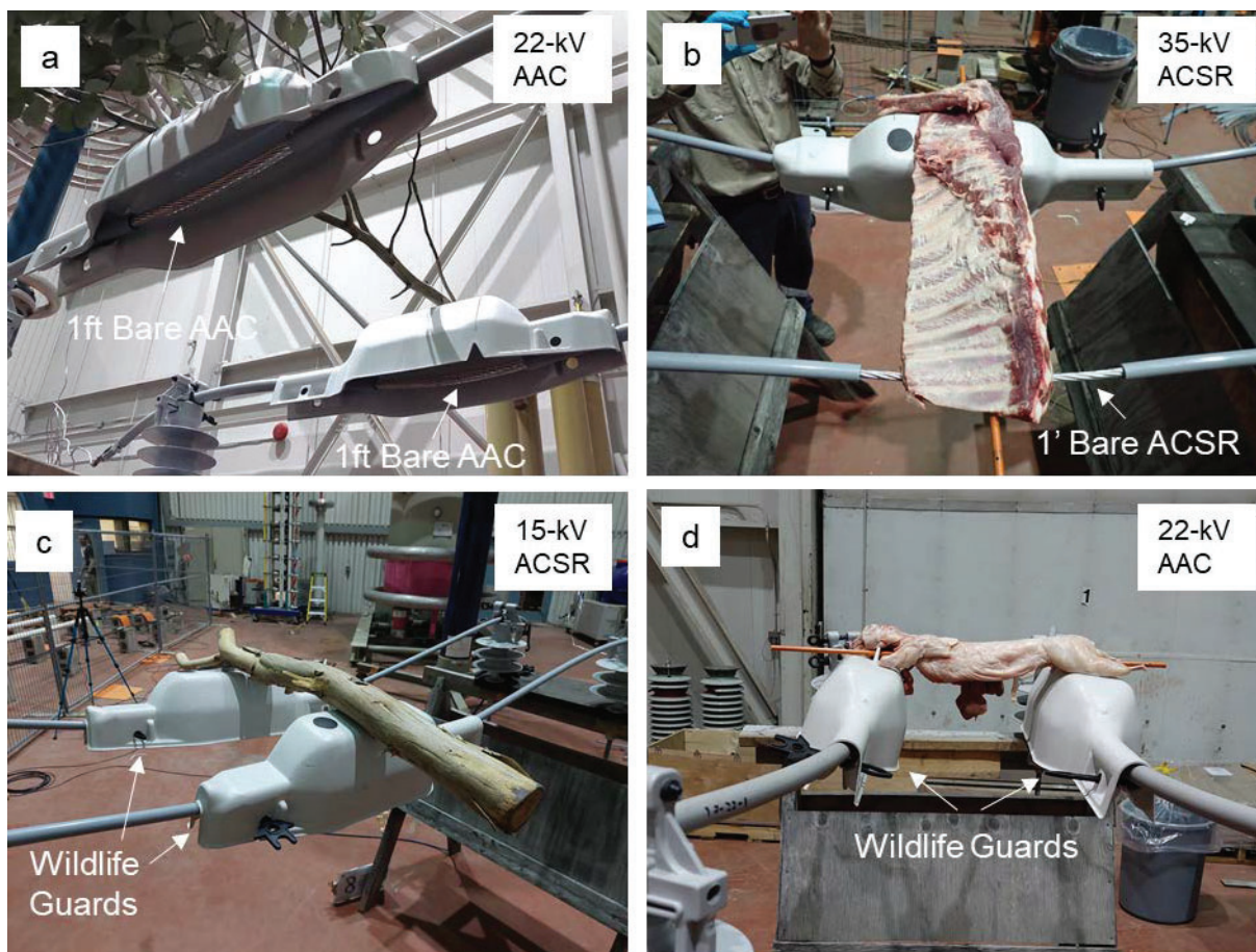
Figure 8. Wildlife guard tests in various configurations at rated voltages. (a) Leafy branches bridging two 22-kV AAC CCs with wildlife guards covering one foot of bare conductor on either side. (b) Simulated animal bridging one 35-kV ACSR CC with a wildlife guard and one 35-kV ACSR CC with one foot of bare conductor exposed. (c) Large eucalyptus stick bridging two 15-kV ACSR CCs with wildlife guards covering one foot of bare conductor on either side. (d) Simulated animal bridging one 22-kV AAC CC with wildlife guards covering one foot of bare conductor on either side.
