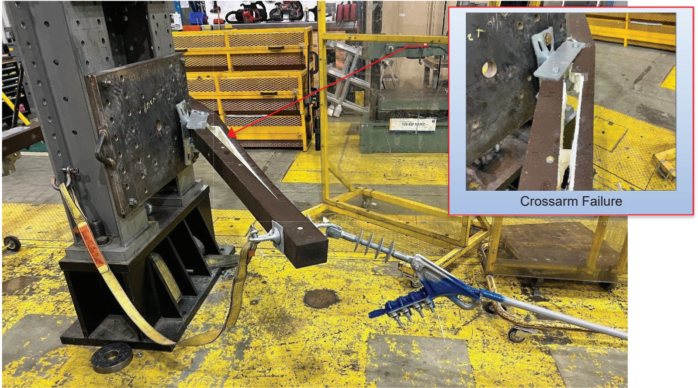
Figure 6-23: Sample 6.2 – Failure Location
