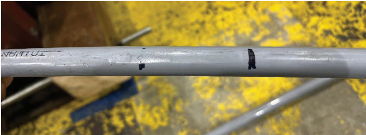
Figure 6-8: [REDACTED] - Typical 1/0 AWG ACSR (17 kV) Conductor Condition after Slip Test
