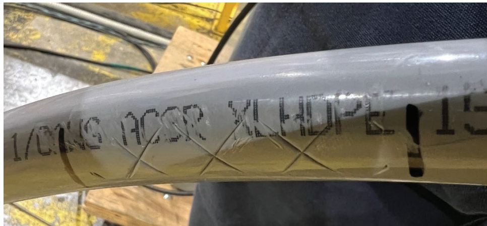
Figure 6-15: Sample 3.2.2 - 35 kV, 1/0 AWG ACSR Condition after Test
