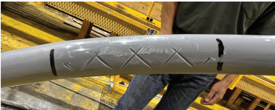
Figure 6-8: Sample 3.1.1 - 17 kV, 1/0 AWG ACSR Condition after Test
