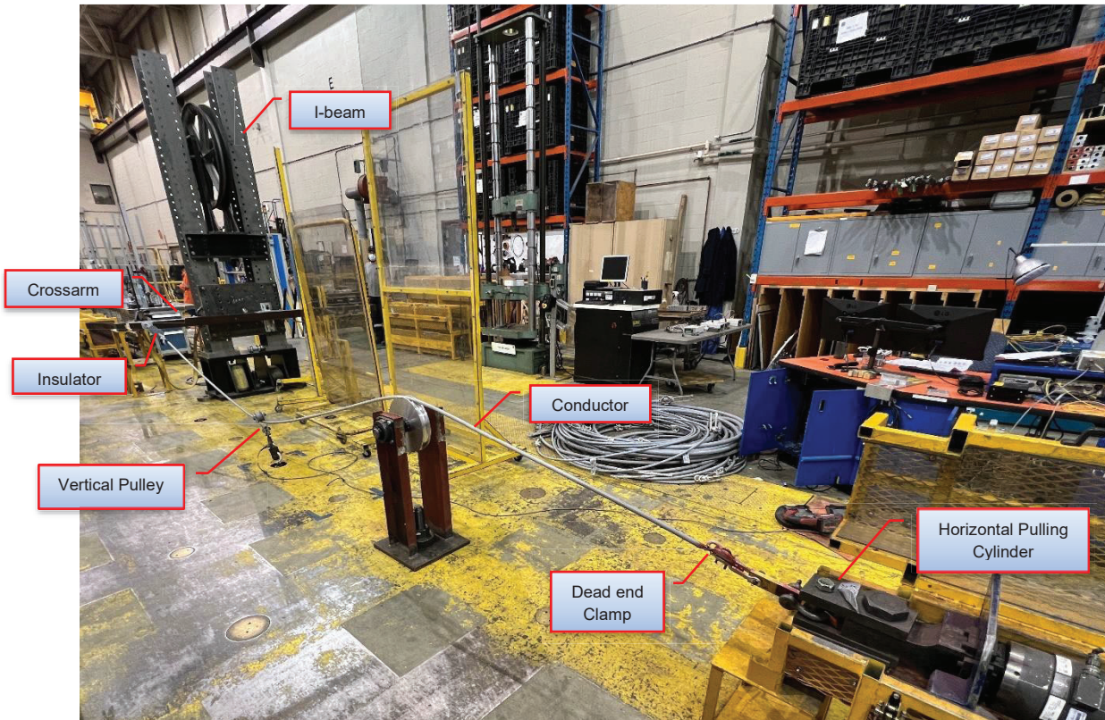
Figure 4-3: Full Mock-up: Picture of the Setup
