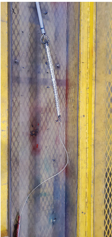
Figure 6-6: Sample 1.1.2 after test (conductor failed at South end of splice)
