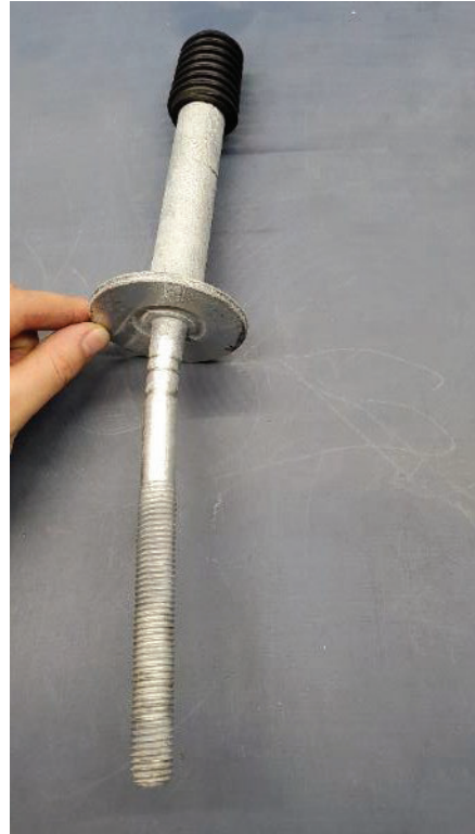
Figure 6-5: [REDACTED] - Typical Bend in Insulator Pin after Slip Test
